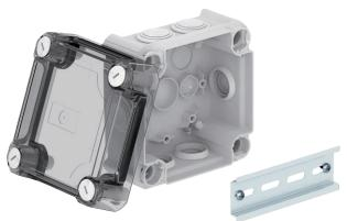
Junction box for the connection of cables and lines indoors and in protected outdoor areas. Square design with plug-in seals to the sides and knock-out entries in the bottom. Suitable for wall and ceiling mounting and on mounting panels. With the option to fasten inside and to mount via the  $\,$ corner domes. High, transparent cover with quick lock, sealable. Made from halogenfree materials.
