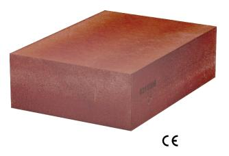
Soft, permanently elastic foam block for cable and combination insulation. Vertical and transverse installation to achieve different fire resistance classes. Can be combined with the two-component fire protection foam PYROSIT® NG. Can be used in solid ceilings and walls and in light-duty partitions and is approved for many installations. CE-labelled construction product according to ETA-15/0803 for applications with fire resistance periods of up to 120 minutes.
