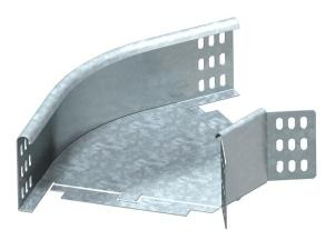
45° bend, horizontal, for all cable tray types of 3" side height. The fitting is shipped in an unmounted state. The WKV 85 angle connector is designed for 90° bends and can be adjusted to 45° on site. Including appropriate fastening material.
