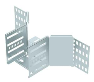
Add-on tee for the creation of a horizontal branch or cross-over, fitting for lock and screw-on cable trays of side height 110 mm. Screwless mounting with double clamps or screw connection with FRS truss-head screws and M6 combination nuts. Can be used in indoor areas. Fastening material must be ordered separately.
