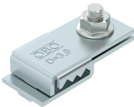
The connection and earthing terminal is used to reduce electrical resistance and therefore improves the electric conductivity in GRM mesh cable systems in the area of the joint. This allows fulfilment of the high demands in terms of the transition resistance according to, for example, NEMA and CSA. Furthermore, the connection and earthing terminal is compulsory when used as a protective conductor in a mesh cable tray system (national regulations have to be followed when creating such a system).
