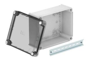
Closed junction box for the connection of cables in indoor and protected outdoor areas. Rectangular design without entries. Suitable for wall and ceiling mounting, on mounting panels and threads in the floor. With the option of fastening inside and to mount via the corner domes. High, transparent cover with quick lock, sealable. Made from halogen-free, UV-resistant materials.
