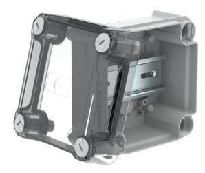
Closed junction box for the connection of cables and lines indoors and in protected outdoor areas. Square design without entries. Suitable for wall and ceiling mounting and on mounting panels. With the option to fasten inside and to mount via the corner domes. High, transparent cover with quick lock, sealable. Made from halogen-free and UV-resistentant materials.
