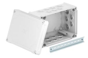
Junction box for the connection of cables and lines indoors and in protected outdoor areas. Rectangular design with plug-in seals. Suitable for wall and ceiling mounting, on mounting panels and threads in the floor. With the option to fasten inside and to mount via the corner domes. High, transparent cover with quick lock, sealable. Made from halogen-free and UV-resistant materials.
