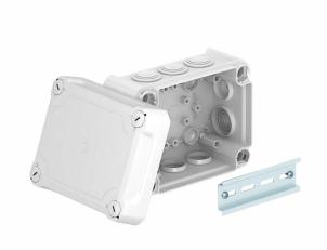
Junction box for the connection of cables and lines indoors and in protected outdoor areas. Rectangular design with plug-in seals to the sides and knock-out entries in the bottom. Suitable for wall and ceiling mounting and on mounting panels. With the option to fasten inside and to mount via the corner domes. High, transparent cover with quick lock, sealable. Made from halogen-free and UV-resistant materials.
