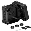
Junction box for the connection of cables and lines indoors and in outdoor areas. Square design with knock-out entries. Suitable for wall and ceiling mounting with the option to fasten outside, inside or to mount via the corner domes. Particularly impact resistant with IK09. Cover with quick lock, sealable. Made from halogen-free and UV-resistant materials.
