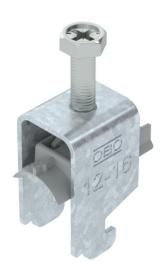
Clamp clip with N-foot, plastic pressure sleeve made of polypropylene. For vertical and horizontal mounting of 2 single cables on a C-profile rail. For slot width 11–12 mm With 1-start screw thread on pressure sleeve, universal hexagonal screw head WAF10, with slot and cross recess. Suitable for assembly indoors and outdoors. Multiple cables should be separated by double sleeves. We recommend the use of a counter-sleeve.
