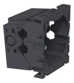
Front locking accessory mounting box for switch systems, with folding, and also removable, base for time-saving cable connection, with feed openings for cable diameters of up to 14 mm. Halogen-free version. Horizontal fixing track 60 mm.
